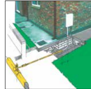
Typical service arrangement
